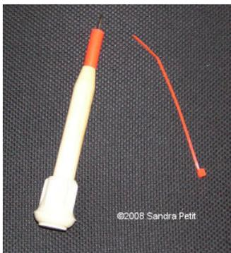
Slip the orange tube onto the pointed end of the awl which is the punching needle. There is no right or wrong side, just slip it on there, all the way to the handle
