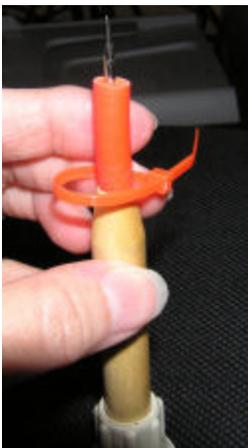
You have to wrap the long tail around the tube. Remember you have the tube placed at the closest point to the handle, furthest from the needle point.
